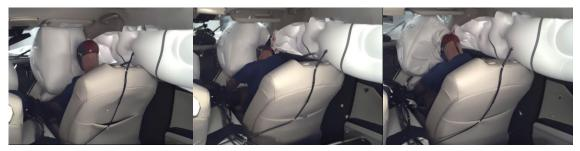
During this crash, the dummy's head briefly loaded the right side of the frontal airbag before contacting the dash through the airbag, though the side curtain helped keep the head on the frontal airbag.
