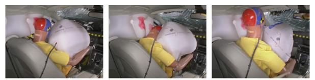
During the crash, the dummy's head briefly loaded the frontal airbag before sliding off the left into a gap between the frontal and side curtain airbags. The frontal airbag was narrow, and there were no other countermeasures to prevent head contact with hard structures forward of the airbag.
