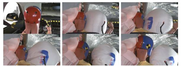
During the crash, the dummy's head loaded the frontal airbag before sliding off the left side. There were no other countermeasures to prevent head contact with hard structures forward of the airbag.
