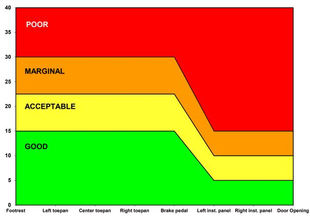
Figure 1 Guidelines for Rating Occupant Compartment Intrusion (cm)
