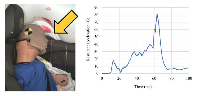
Figure 2 Example of marginal head protection
