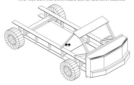
The deformable element has a width of 1,676 mm, a height of 759 mm, and a ground clearance of 379 mm when mounted on the test cart (Figure 3). Detailed information on the IIHS barrier development and evaluation testing has been documented previously (Arbelaez et al., 2002). The IIHS deformable barrier design and performance criteria are documented in the *Side Impact Moving Deformable Barrier Specification* (IIHS, 2007).
